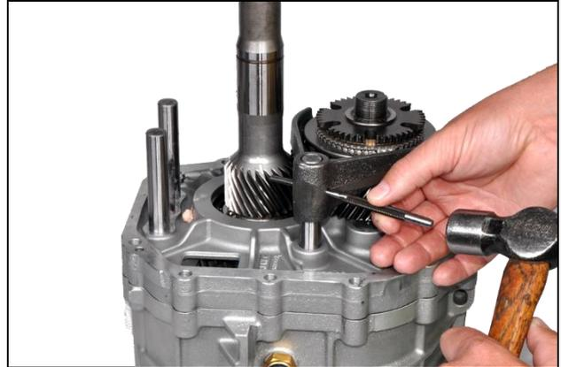
**3.23:** Remove 5<sup>th</sup> gear fork roll pin
