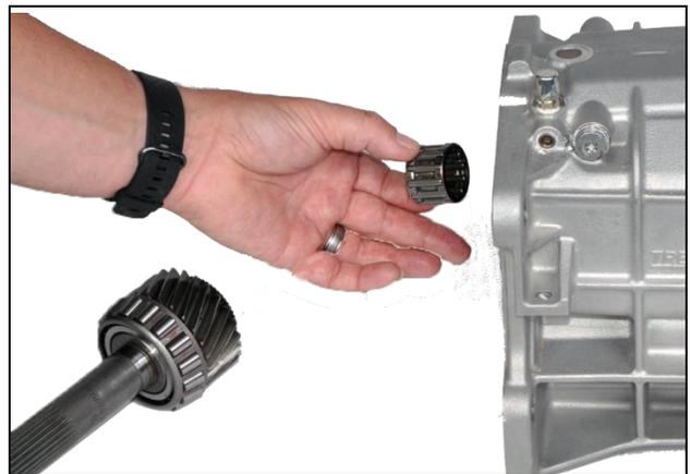
**8.28:** Install input shaft and pocket bearing
