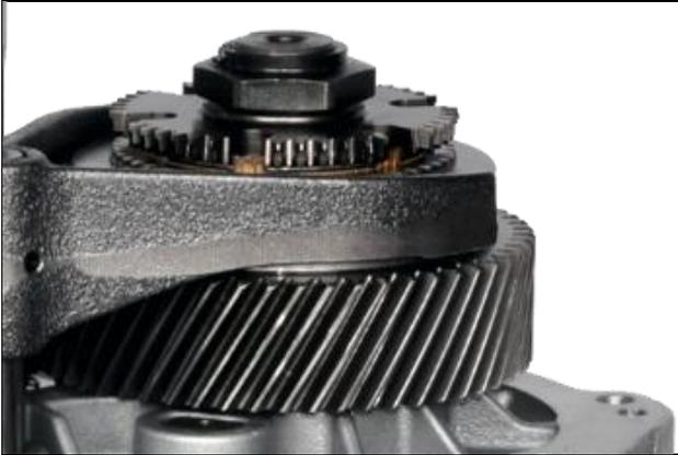
**8.21:** Install counter shaft locking nut
