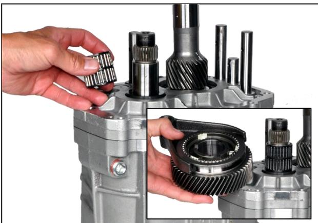
**8.18:** Install 5<sup>th</sup> gear bearing to cluster shaft
