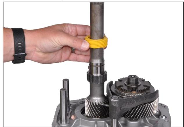
**3.19:** Remove mechanical speedometer gear
