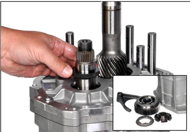
**3.27:** Remove 5<sup>th</sup> gear thrust washer
