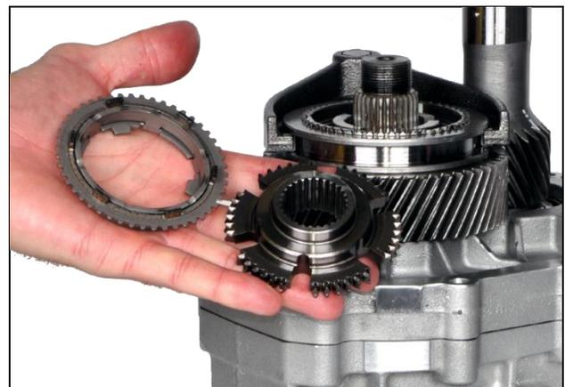
**8.20:** Install 5<sup>th</sup> gear inner and outer blocking rings
