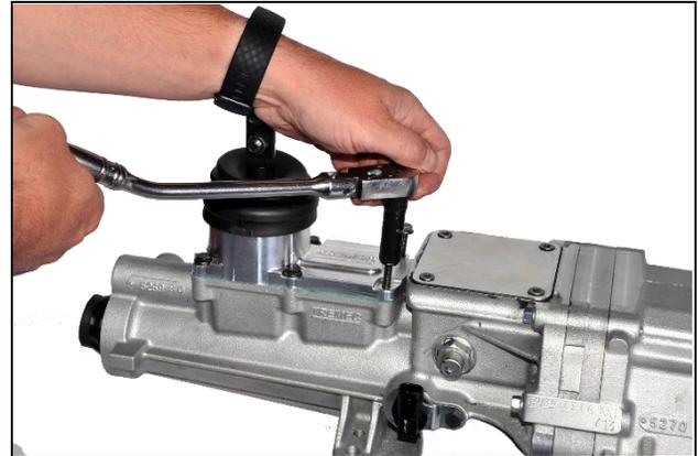
**3.3:** Remove six shift housing mounting bolts
