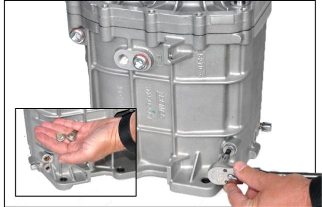
**3.38:** Remove two shift rail detent plugs
