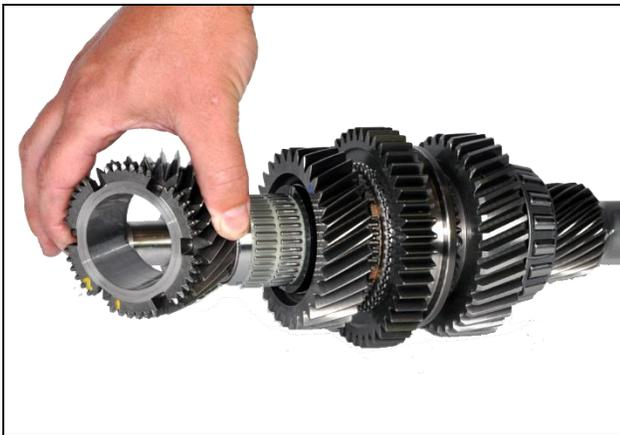
**6.15:** Install 3<sup>rd</sup> gear onto main shaft
