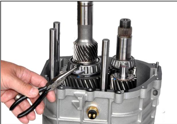
**3.32:** Remove snap ring from 5<sup>th</sup> reverse selector link inside main case
