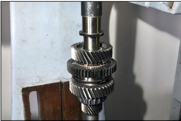
**6.13:** Press 3<sup>rd</sup> gear thrust washer and bearing journal onto main shaft
