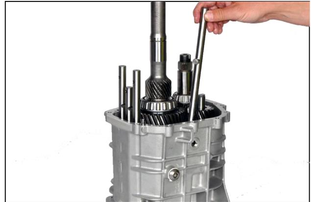
**8.10:** Install 5<sup>th</sup> reverse shift rail into case (Note: Rail detent roller fits in selector arm)
