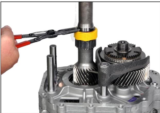
**3.18:** Remove speedometer gear snap ring
