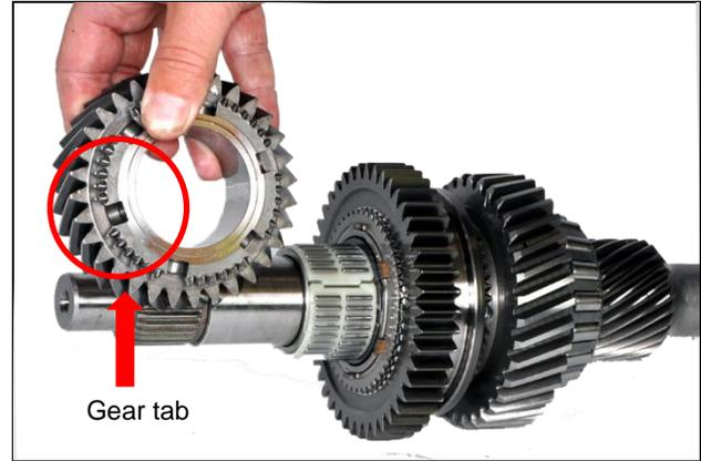
**6.12:** Install 2<sup>nd</sup> gear onto main shaft. Be careful to line up blockers into gear tabs
