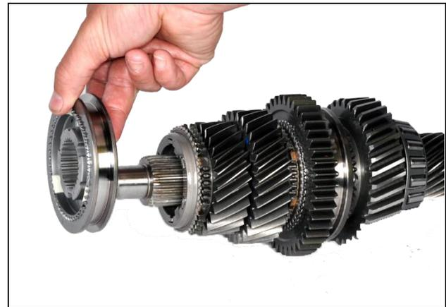
**6.16:** Install 3<sup>rd</sup> gear blocking ring
