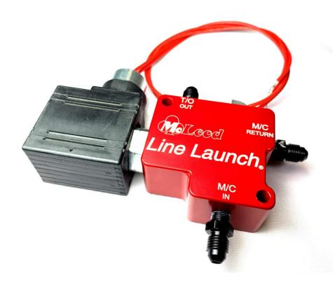
2) Route a line from the clutch master cylinder to the inlet on the Line Launch (M/C IN). Route another line from the Line Launch (M/C RETURN) to the master cylinder reservoir. Route a line from the (SLAVE OUT) port to the hydraulic slave cylinder (This may be the existing line). Tighten all
