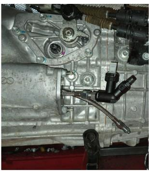
31. Connect lines to the McLeod bearing. The shorter line connects to the bottom of the bearing and the longer line connect to the top and is the line to install the bleeder screw into.
