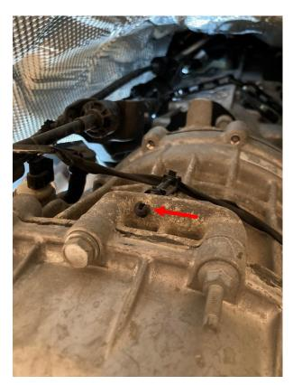
16. Remove the upper shift cable from the bracket. The cable can be disconnected from the bracket by pulling on the front side of the cable retainer (spring loaded). Leave the cable connected to the transmission/transfer case, but slide it out of the bracket. **Do not bend** or kink the shift cables. **Do not allow the transmission to hang on the shift cables.**
