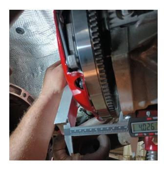
29. Slide the new hydraulic slave bearing onto the transmission bearing retainer (use light grease or lube on the o-rings) and measure from the transmission face to the slave bearing. Adjust the bearing by turning it, clockwise to increase the number and counter clockwise to decrease the number, until the measurement from the bearing to the bellhousing face matches the number calculated in the previous step.
