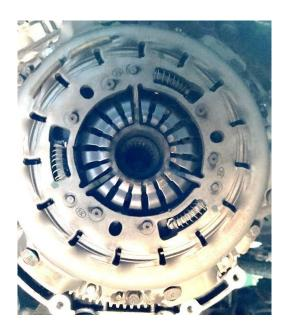
25. Remove the eight flywheel bolts with a T50 TORX and remove the flywheel.
