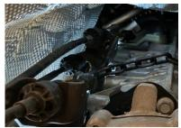
17. Disconnect plug for the sensor in the rear of the transfer case.
