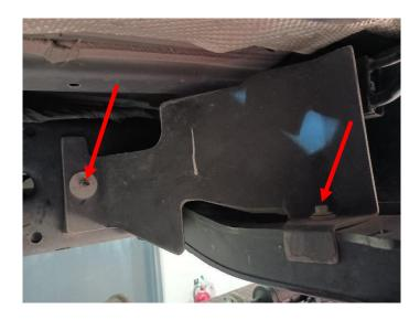
9. Remove the 6 bolts attaching the skid plate.
