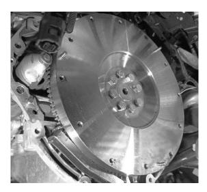
27. Install clutch and pressure plate using the clutch alignment tool and the fasteners provided and torque to 25 ft lbs.
