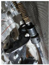
5. Remove the 2 bolts holding the fuel line on the right side of the transmission.
