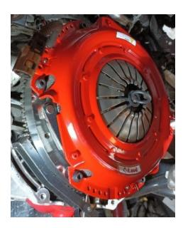
28. Using a straight edge measure from clutch fingers to engine block, taking care make sure the straight edge is even. Use this measurement and add 0.300. For reference this clutch setup measured 4.026 in.
