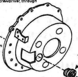
1. PIVOT BASE — Screw in tight — flush with bell housing
