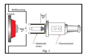
Measure and record your "A" dimension from the transmissions mounting surface to the tip of the pressure plate finger when clutch is fully installed and torqued down.
